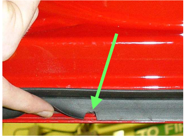
figure 3 - Cut notch in weather seal as shown
