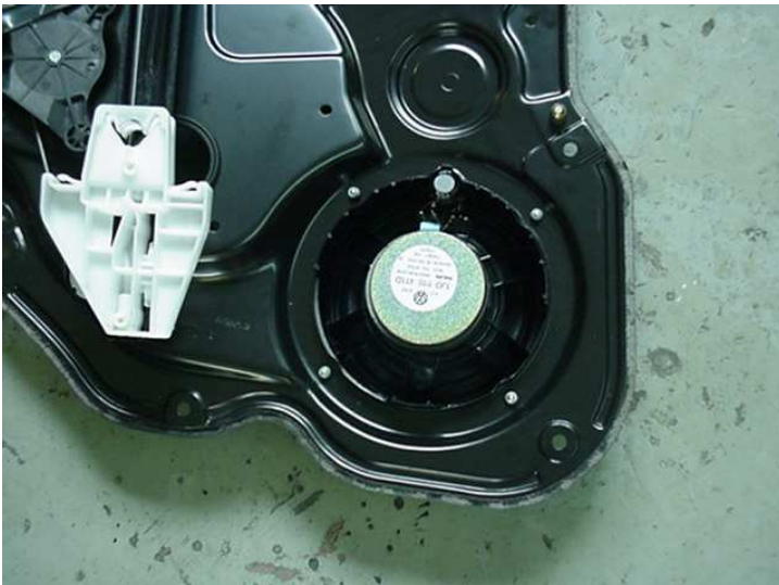
figure 4 - Remove old seal from ancillaries carrier
