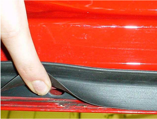
figure 2 - Outer weather seal on door - (view from below)
