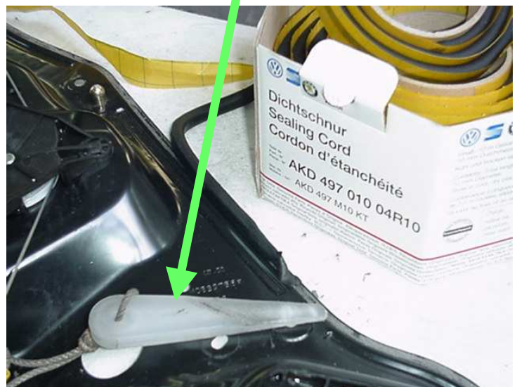
figure 5 - Replace seal with sealing cord
